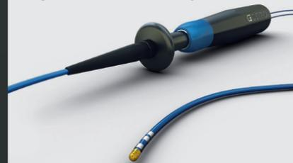
The Flex-to-Rigid (F2R) miniature assembly platform is designed to bring complex electronic sensing functionality to the tip of smart catheters. (<http://informed-project.eu/downloads/F2R.pdf>)
