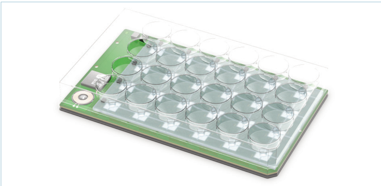
Figure 6 An impression of the smart well plate that is currently being developed in the ECSEL JU project Moore4Medical. It is designed to bring the organ-on-chip devices of different manufacturers in a standard format.
